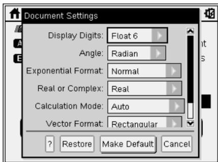
3. Press **tab** to move through the list of settings. Press **▲** to move backward through the list.
