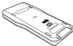
2. Turn the handheld top side up, and slide the keypad away from the display screen.
